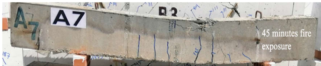
a) Experimental A7 beam cracking pattern
