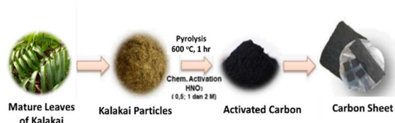
Figure 1. Synthesis mechanism of activated carbon sheet from Kalakai.
