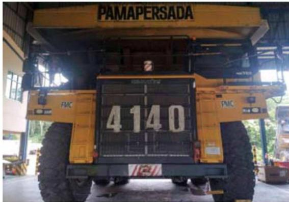
Gambar 1 Unit dump truck HD 785-7 Komatsu
